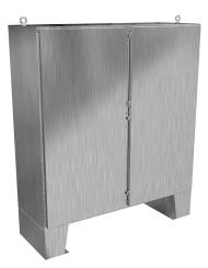
Hammond enclosure, NEMA 3R/4/4X/12/13, 72 x 72 x 24in (HxWxD), floor mount, 316 stainless steel, #4 brush finish, 2-door, stainless steel clamps, padlock hasp and staple.
