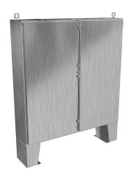
Hammond enclosure, NEMA 3R/4/4X/12/13, 60 x 60 x 12in (HxWxD), floor mount, 316 stainless steel, #4 brush finish, 2-door, stainless steel clamps, padlock hasp and staple.
