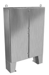
Hammond enclosure, NEMA 3R/4/4X/12/13, 60 x 48 x 12in (HxWxD), floor mount, 316 stainless steel, #4 brush finish, 2-door, stainless steel clamps, padlock hasp and staple.
