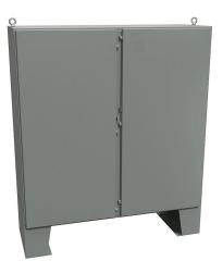
Hammond enclosure, NEMA 3R/4/12/13, 72 x 72 x 24in (HxWxD), floor mount, carbon steel, ANSI 61 gray, powder coat finish, 2-door, stainless steel clamps, padlock hasp and staple.
