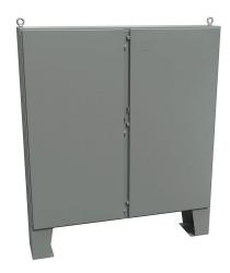
Hammond enclosure, NEMA 3R/4/12/13, 72 x 72 x 12in (HxWxD), floor mount, carbon steel, ANSI 61 gray, powder coat finish, 2-door, stainless steel clamps, padlock hasp and staple.
