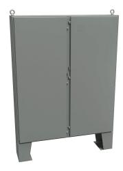
Hammond enclosure, NEMA 3R/4/12/13, 72 x 60 x 12in (HxWxD), floor mount, carbon steel, ANSI 61 gray, powder coat finish, 2-door, stainless steel clamps, padlock hasp and staple.
