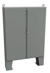
Hammond enclosure, NEMA 3R/4/12/13, 60 x 48 x 10in (HxWxD), floor mount, carbon steel, ANSI 61 gray, powder coat finish, 2-door, stainless steel clamps, padlock hasp and staple.
