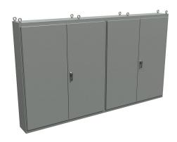
Hammond enclosure, NEMA 12, 86 x 149 x 14in (HxWxD), freestanding, carbon steel, ANSI 61 gray, powder coat finish, 4-door, 3-point keylocking handle.
