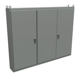
Hammond enclosure, NEMA 12, 86 x 112 x 14in (HxWxD), freestanding, carbon steel, ANSI 61 gray, powder coat finish, 3-door, 3-point keylocking handle.
