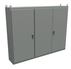
Hammond enclosure, NEMA 12, 86 x 112 x 20in (HxWxD), freestanding, carbon steel, ANSI 61 gray, powder coat finish, 3-door, 3-point keylocking handle.
