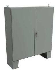
Hammond enclosure, NEMA 12, 72 x 72 x 20in (HxWxD), floor mount, carbon steel, ANSI 61 gray, powder coat finish, doubledoor, 3-point keylocking handle.
