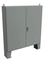
Hammond enclosure, NEMA 12, 72 x 72 x 12in (HxWxD), floor mount, carbon steel, ANSI 61 gray, powder coat finish, double-door, 3-point keylocking handle.
