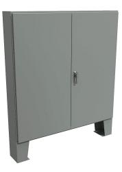
Hammond enclosure, NEMA 12, 72 x 72 x 10in (HxWxD), floor mount, carbon steel, ANSI 61 gray, powder coat finish, double-door, 3-point keylocking handle.
