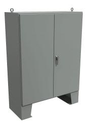
Hammond enclosure, NEMA 12, 72 x 60 x 24in (HxWxD), floor mount, carbon steel, ANSI 61 gray, powder coat finish, double-door, 3-point keylocking handle.
