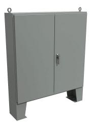
Hammond enclosure, NEMA 12, 60 x 60 x 12in (HxWxD), floor mount, carbon steel, ANSI 61 gray, powder coat finish, double-door, 3-point keylocking handle.
