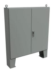
Hammond enclosure, NEMA 12, 60 x 60 x 10in (HxWxD), floor mount, carbon steel, ANSI 61 gray, powder coat finish, doubledoor, 3-point keylocking handle.
