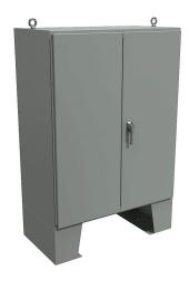
Hammond enclosure, NEMA 12, 60 x 48 x 24in (HxWxD), floor mount, carbon steel, ANSI 61 gray, powder coat finish, doubledoor, 3-point keylocking handle.
