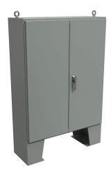
Hammond enclosure, NEMA 12, 60 x 48 x 16in (HxWxD), floor mount, carbon steel, ANSI 61 gray, powder coat finish, doubledoor, 3-point keylocking handle.
