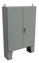
Hammond enclosure, NEMA 12, 60 x 48 x 12in (HxWxD), floor mount, carbon steel, ANSI 61 gray, powder coat finish, double-door, 3-point keylocking handle.
