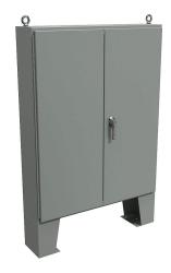
Hammond enclosure, NEMA 12, 60 x 48 x 10in (HxWxD), floor mount, carbon steel, ANSI 61 gray, powder coat finish, doubledoor, 3-point keylocking handle.
