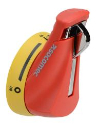
Socomec rotary handle, pistol, S1, heavy duty metallic hasp, red/ yellow, external right side mount, 2-position, lockable in OFF only, NEMA 4/4X.
