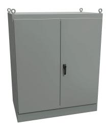
Hammond enclosure, NEMA 12, 72 x 60 x 36in (HxWxD), freestanding, carbon steel, ANSI 61 gray, powder coat finish, double-door, 3-point keylocking handle.
