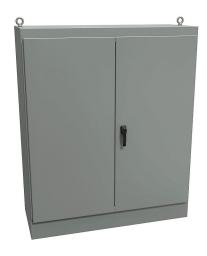
Hammond enclosure, NEMA 12, 72 x 60 x 24in (HxWxD), freestanding, carbon steel, ANSI 61 gray, powder coat finish, double-door, 3-point keylocking handle.
