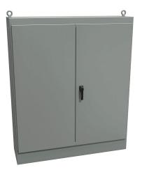
Hammond enclosure, NEMA 12, 72 x 60 x 18in (HxWxD), freestanding, carbon steel, ANSI 61 gray, powder coat finish, double-door, 3-point keylocking handle.
