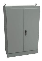
Hammond enclosure, NEMA 12, 72 x 48 x 24in (HxWxD), freestanding, dual access, carbon steel, ANSI 61 gray, powder coat finish, double-door, 3-point keylocking handle.
