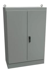
Hammond enclosure, NEMA 12, 72 x 48 x 24in (HxWxD), freestanding, carbon steel, ANSI 61 gray, powder coat finish, double-door, 3-point keylocking handle.
