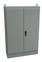
Hammond enclosure, NEMA 12, 72 x 48 x 18in (HxWxD), freestanding, carbon steel, ANSI 61 gray, powder coat finish, double-door, 3-point keylocking handle.
