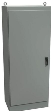
Hammond enclosure, NEMA 12, 90 x 36 x 24in (HxWxD), freestanding, dual access, carbon steel, ANSI 61 gray, powder coat finish, single-door, 3-point keylocking handle.
