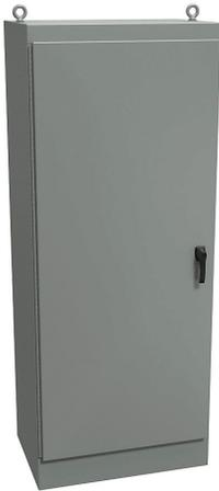
Hammond enclosure, NEMA 12, 90 x 36 x 24in (HxWxD), freestanding, carbon steel, ANSI 61 gray, powder coat finish, single-door, 3-point keylocking handle.
