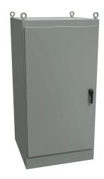
Hammond enclosure, NEMA 12, 72 x 36 x 36in (HxWxD), freestanding, carbon steel, ANSI 61 gray, powder coat finish, single-door, 3-point keylocking handle.
