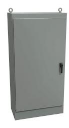
Hammond enclosure, NEMA 12, 72 x 36 x 18in (HxWxD), freestanding, carbon steel, ANSI 61 gray, powder coat finish, single-door, 3-point keylocking handle.
