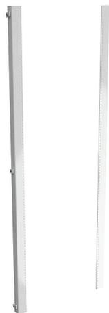
Hammond enclosure rack mounting angle, carbon steel, full-height mount, RAL 9003 white, powder coat finish. Package of 2. For use with 72x24in (HxW) freestanding enclosures. For mounting 19in rack equipment. Drilled and tapped 10-32 to EIA spacing.
