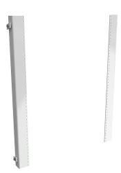
Hammond enclosure rack mounting angle, carbon steel, halfheight mount, RAL 9003 white, powder coat finish. Package of 2. For use with 60x24in (HxW) freestanding enclosures. For mounting 19in rack equipment. Drilled and tapped 10-32 to EIA spacing.
