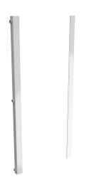
Hammond enclosure rack mounting angle, carbon steel, fullheight mount, RAL 9003 white, powder coat finish. Package of 2. For use with 60x24in (HxW) freestanding enclosures. For mounting 19in rack equipment. Drilled and tapped 10-32 to EIA spacing.
