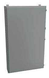
Hammond enclosure, NEMA 12/13, 60 x 36 x 8in (HxWxD), wall mount, carbon steel, ANSI 61 gray, powder coat finish, single-door, stainless steel clamps, padlock hasp and staple.
