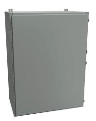
Hammond enclosure, NEMA 12/13, 48 x 36 x 20in (HxWxD), wall mount, carbon steel, ANSI 61 gray, powder coat finish, single-door, stainless steel clamps, padlock hasp and staple.
