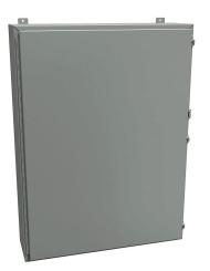
Hammond enclosure, NEMA 12/13, 48 x 36 x 10in (HxWxD), wall mount, carbon steel, ANSI 61 gray, powder coat finish, single-door, stainless steel clamps, padlock hasp and staple.
