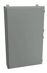
Hammond enclosure, NEMA 12/13, 48 x 30 x 8in (HxWxD), wall mount, carbon steel, ANSI 61 gray, powder coat finish, single-door, stainless steel clamps, padlock hasp and staple.
