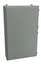
Hammond enclosure, NEMA 12/13, 48 x 30 x 10in (HxWxD), wall mount, carbon steel, ANSI 61 gray, powder coat finish, single-door, stainless steel clamps, padlock hasp and staple.
