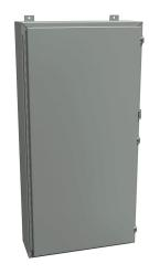
Hammond enclosure, NEMA 12/13, 48 x 24 x 8in (HxWxD), wall mount, carbon steel, ANSI 61 gray, powder coat finish, single-door, stainless steel clamps, padlock hasp and staple.
