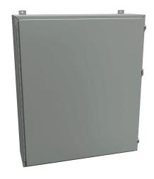
Hammond enclosure, NEMA 12/13, 42 x 36 x 10in (HxWxD), wall mount, carbon steel, ANSI 61 gray, powder coat finish, single-door, stainless steel clamps, padlock hasp and staple.
