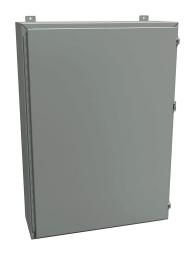
Hammond enclosure, NEMA 12/13,  $42 \times 30 \times 10$ in (HxWxD), wall mount, carbon steel, ANSI 61 gray, powder coat finish, singledoor, stainless steel clamps, padlock hasp and staple.
