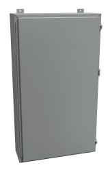
Hammond enclosure, NEMA 12/13, 42 x 24 x 8in (HxWxD), wall mount, carbon steel, ANSI 61 gray, powder coat finish, single-door, stainless steel clamps, padlock hasp and staple.
