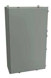
Hammond enclosure, NEMA 3R/4/12, 60 x 36 x 16in (HxWxD), wall mount, carbon steel, ANSI 61 gray, powder coat finish, single-door, stainless steel clamps, padlock hasp and staple.
