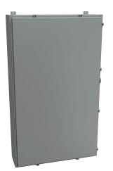
Hammond enclosure, NEMA 3R/4/12, 60 x 36 x 10in (HxWxD), wall mount, carbon steel, ANSI 61 gray, powder coat finish, single-door, stainless steel clamps, padlock hasp and staple.
