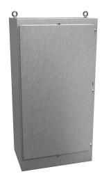
Hammond enclosure, NEMA 3R/4/4X/12/13, 72 x 36 x 24in (HxWxD), freestanding, 304 stainless steel, #4 brush finish, single-door, stainless steel clamps, padlock hasp and staple.
