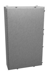
Hammond enclosure, NEMA 3R/4/4X/12/13, 60 x 36 x 12in (HxWxD), wall mount, 304 stainless steel, #4 brush finish, single-door, stainless steel clamps, padlock hasp and staple.
