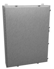
Hammond enclosure, NEMA 3R/4/4X/12/13, 48 x 36 x 8in (HxWxD), wall mount, 304 stainless steel, #4 brush finish, single-door, stainless steel clamps, padlock hasp and staple.
