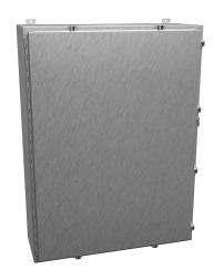
Hammond enclosure, NEMA 3R/4/4X/12/13, 48 x 36 x 12in (HxWxD), wall mount, 304 stainless steel, #4 brush finish, single-door, stainless steel clamps, padlock hasp and staple.
