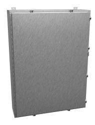
Hammond enclosure, NEMA 3R/4/4X/12/13, 48 x 36 x 10in (HxWxD), wall mount, 304 stainless steel, #4 brush finish, single-door, stainless steel clamps, padlock hasp and staple.
